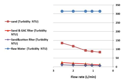
Figure 8. Variation of turbidity with flow rate of treated and raw storm water
