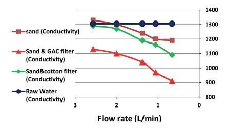
Figure 6. Variation of conductivity with flow rate of treated and raw storm water
